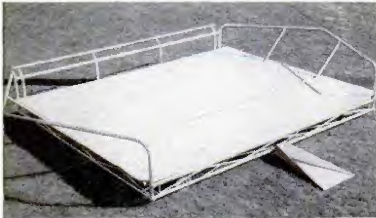
Welded-steel electrical conduit forms frame of the pit. The box into which the pole end fits is detached for high jumping
